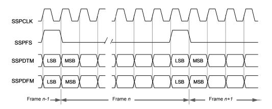
Figure 5.10-3 PCM Frame format for a continuous transfer
